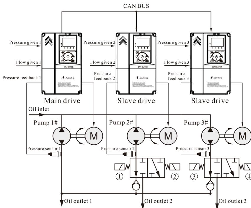
Diagram I-2 Multi-pump splitting flow structure diagram
