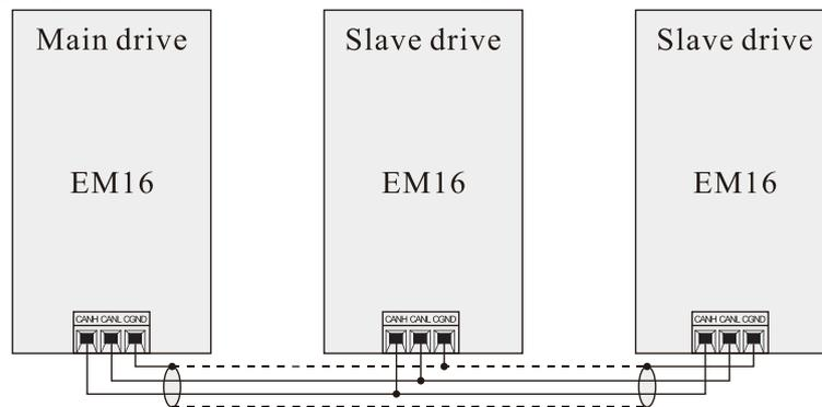
Diagram I-3 CAN bus connection diagram
