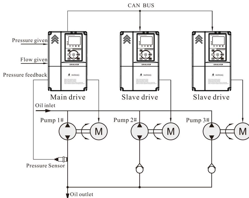
Diagram I-1 Multi-pump combining flow structure diagram
