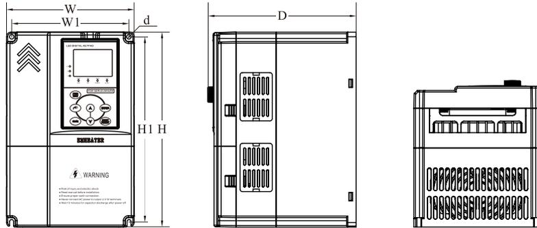
Diagram 2-3 Single phase 4~22kW Wall-mounted installation dimensions
