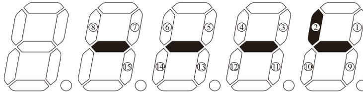
Diagram I-12 H2-05 Slave pump address setting
