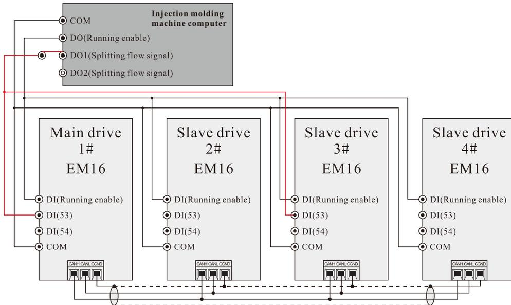
Diagram I-11 2+2 combined splitting flow control
