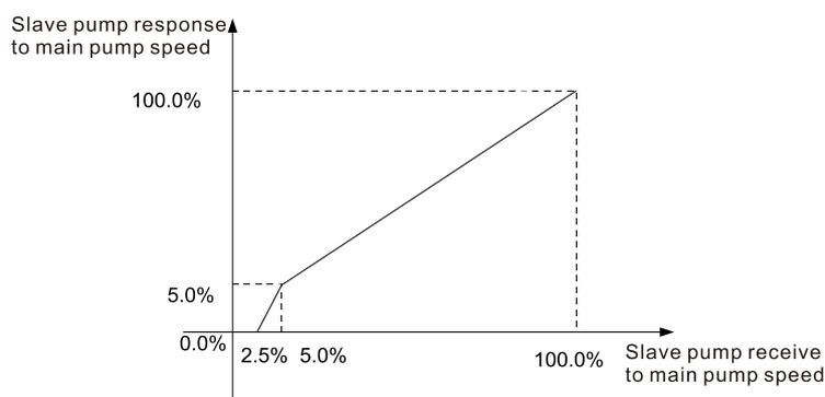
Diagram I-4 Slave pump response to main pump speed command diagram
