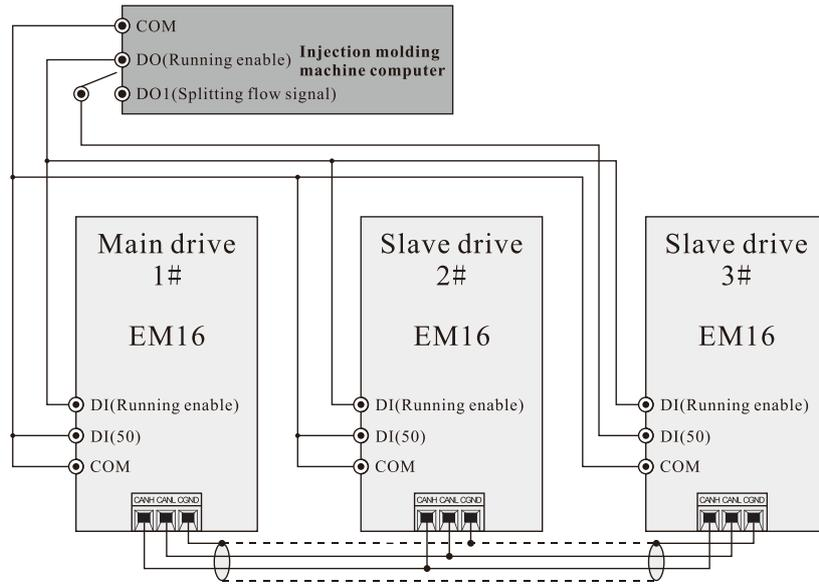
Diagram I-8 2+1 combined splitting flow control
