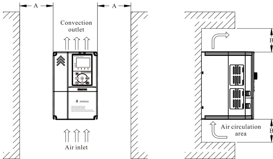
Diagram3-1 Ventilating duct installation dimension diagram of servo drive
