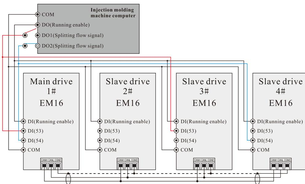
Diagram I-14 3+13+1 combined splitting flow control
