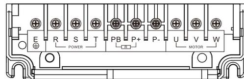
Note: P + and P- are DC input, prohibit external braking unit
