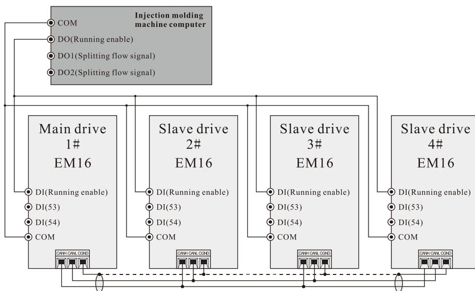
Diagram I-9 4 pump combining flow control
