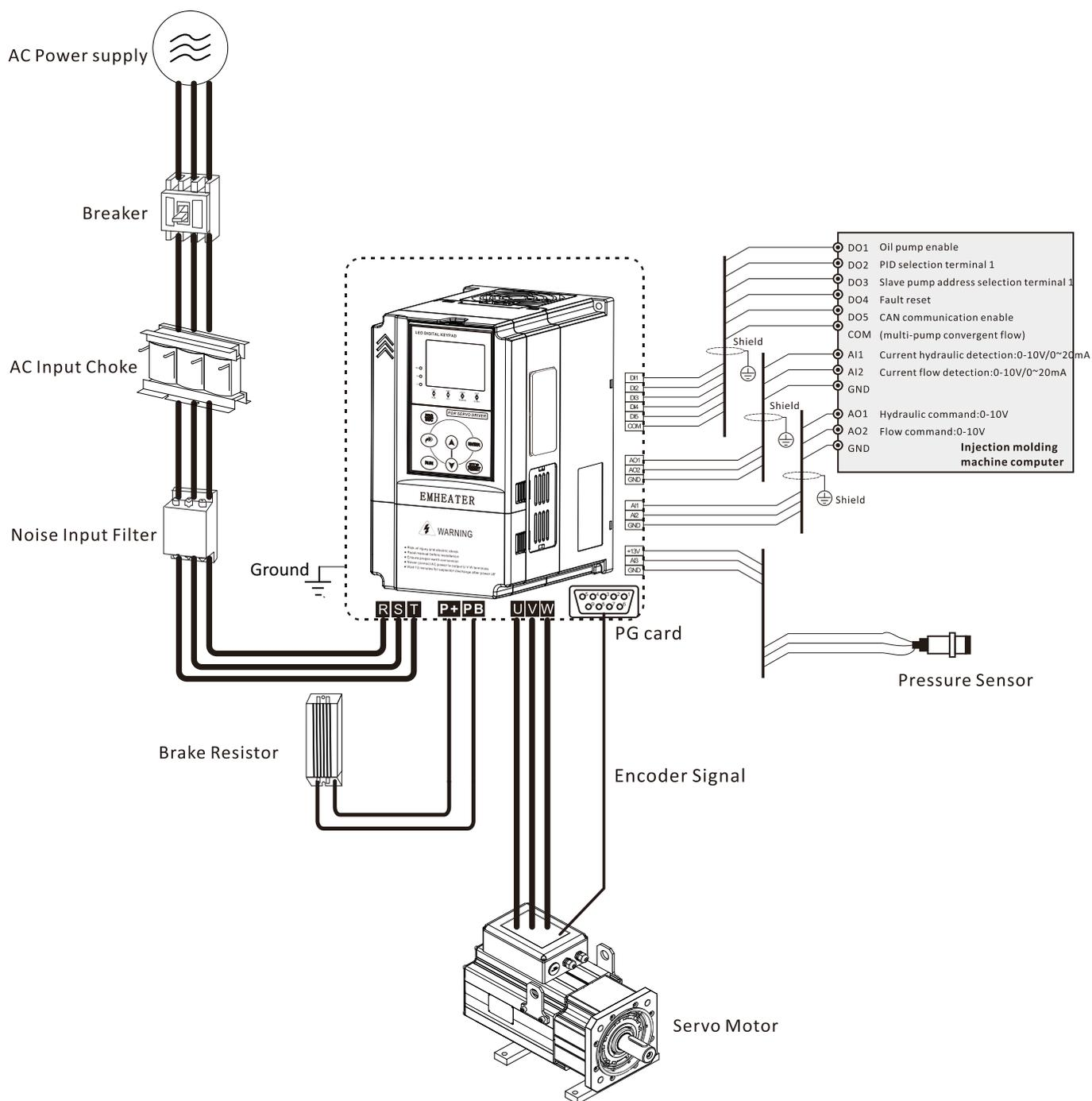
Diagram 3-2 Peripheral Devices Connection
