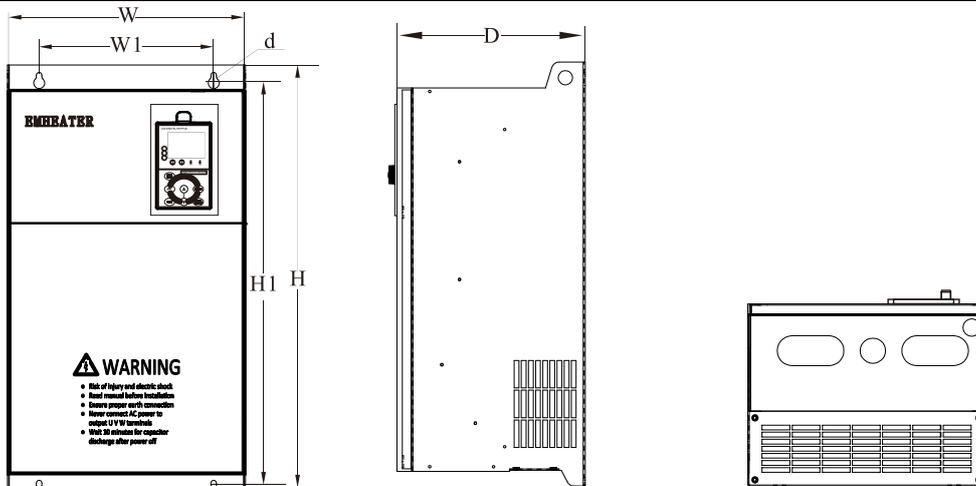
Diagram 2-4 Three phase 30~90kW Wall-mounted installation dimensions
