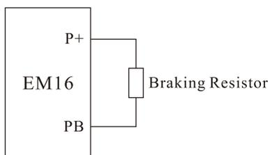
Diagram 2-5 Braking resistor connection scheme
